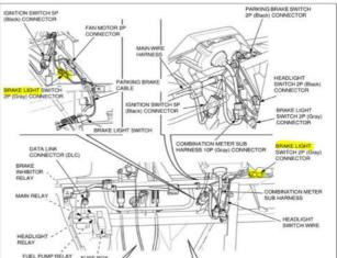
Note: - This photo is from another vehicle but shows the older style of brake switch plug (the grey plugs).
