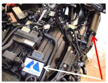
This photo shows the bike with the air filter housing removed, looking down at the area in front of the throttle bodies.
